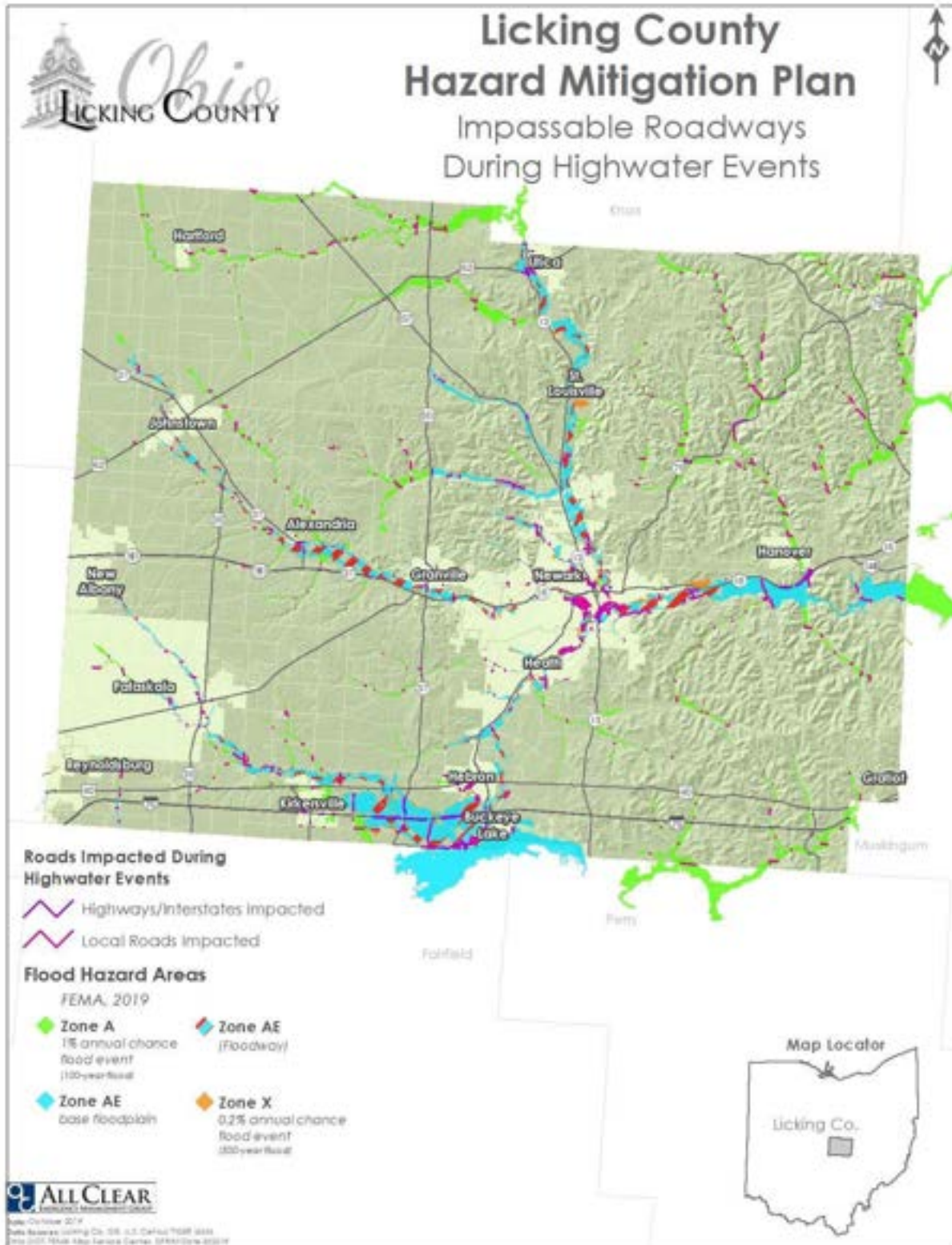
Figure 51: Impassable Roadways During Highwater Events
